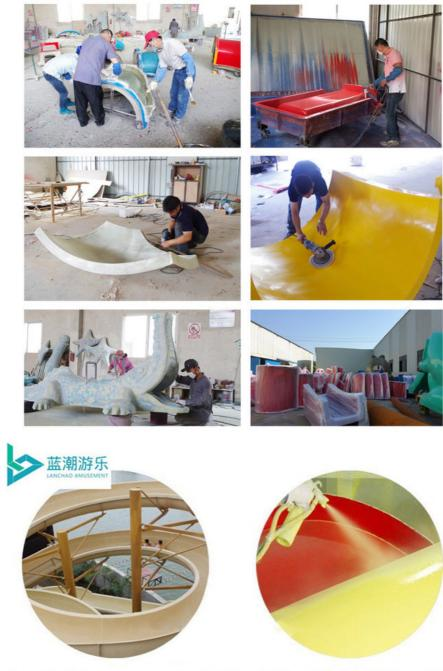
Using the high-performance material of Fiber Reinforced Plastics/FRP featured in strong toughness, long-term aging resistance and safety. Employed the special gel-coat on the slide surface with the function of high-mech anic strength, smooth, anti-high temperature/-corrosion/-oxidant/-UV/-fading.
