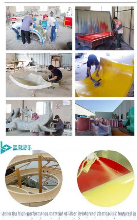
Using the high-performance material of Elber Beinforced Plastics/FBP featured in Employed the special gel-coat on the slide surface with the function of high-mech
