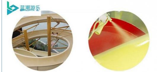
Using the high-performance material of Eiher Beinforced Plastics/FBP featured in Employed the special gel-coat on the slide surface with the function of high-mech
